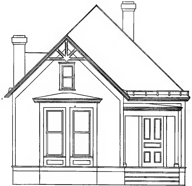
Fig. 12.—The Front Elevation Partially Finished.—Scale, \frac{1}{8} Inch to the Foot.
